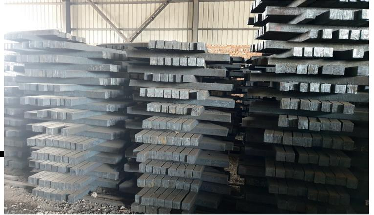
*The billet is HOT ROLLED to the Y bar profile required, straightened and cut to length*
